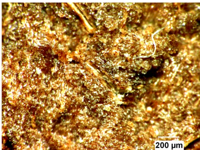
Fig. 10. Micrograph of a fresh broken surface in the soft wooden region normal to the macadamia outer hardshell, showing most bundles of fibres ending here and the occurrence of domains.
