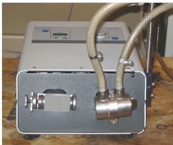
Figure 10: Lab-size vibration ball-mill: 20 ml beakers with temperature control (-78 to 100°C) for initial tests (do not use planetary mills) [23].
