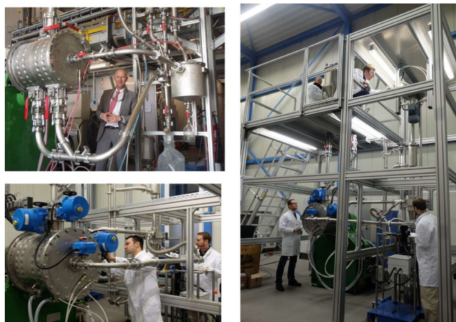
Figure 14: Different 100 L Simoloyer® ball-mills and Auto-batch-operation (continuous production). We thank the Zoz-Group Ltd. Wenden, Germany for permission to present these images.
